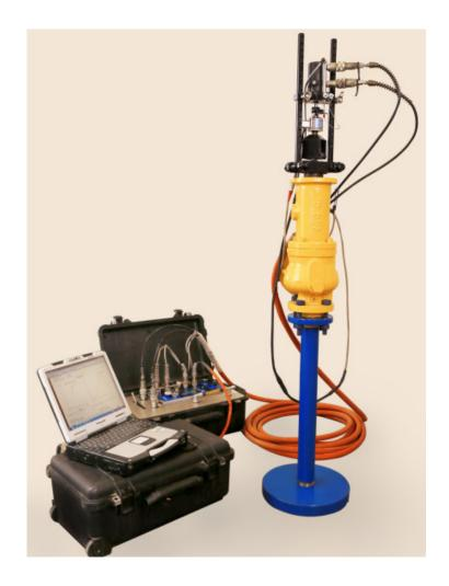
The Uni-Test is more accurate than a cold test on a bench, as the tests are executed under normal operating condition of the valve. Moreover, as the valves are tested in-situ, costs associated with a shutdown, removal and the risk of damage during the transportation are all avoided.
