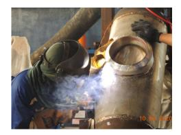
Wellube manufactures specialised hot tap/line fittings in-house based on client requirements in line with the ASME codes. As a complete turnkey service, we also have a team of certified in-service welders available to meet the wide and varied requirements of customers.
