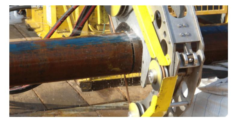
All our diamond wire saws are designed to give you maximum cutting range flexibility with the smallest footprint and the cutting frame can be configured in multiple ways, depending on, for example, the direction of cut, or the size and shape of items to be cut. The wire travels through the driving pulleys at high speed, whilst appropriate angulation and proper tension provides the necessary cutting friction.
