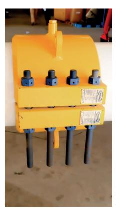
The SSRC consists of two halves which are joined by means of nearly tangential bolting, to produce a high integrity pressure vessel around the affected area of the damaged pipeline. Primary sealing is provided by the highest quality moulded elastomer seals, selected for their compatibility with the pipeline's product, environment and operating temperature range.
